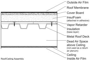
To determine the dew point temperature for a given assembly, the interior temperature and relative humidity must be known. Respectively, these values are also commonly referred to as design temperature and design relative humidity.
